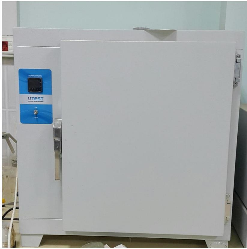
This oven have been designed for drying asphalt, soil, rock, concrete, aggregate or similar materials. 50, 120, 250, 500 and 750 liter capacity models are available. Temperature range is from ambient to 200°C. The interior is manufactured from stainless steel and the exterior is robustly constructed from sheet steel finished in powder coated paint.
