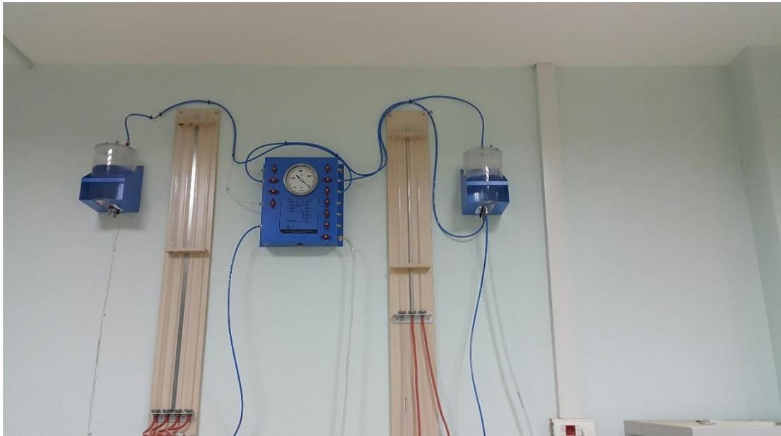
Constant Head Permeability Set are used to study the behaviour of soil, relatively coarse-grained soil such as sands and gravel, in its natural conditions with respect to water flow.
