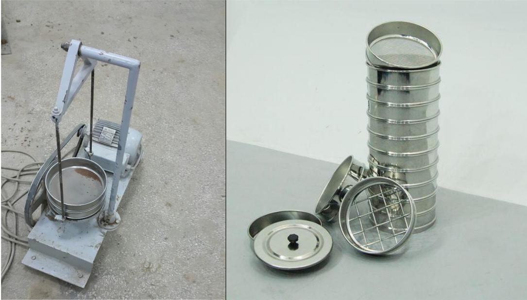
This sieve shaker is fitted with a very efficient clamping device that ensures sieves are held firmly without over-tightening and allows them to be quickly removed and replaced
