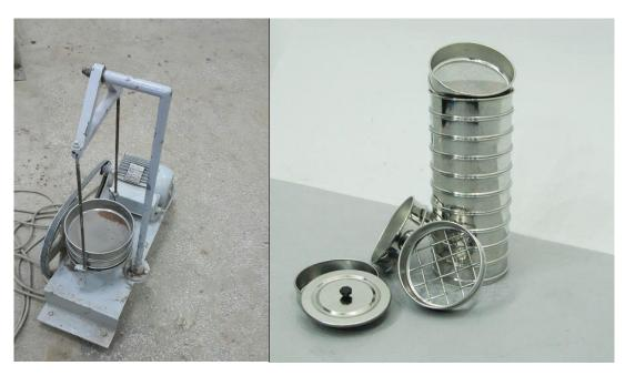
This sieve shaker is fitted with a very efficient clamping device that ensures sieves are held firmly without over-tightening and allows them to be quickly removed and replaced
