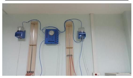
Constant Head Permeability Set are used to study the behaviour of soil, relatively coarse-grained soil such as sands and gravel, in its natural conditions with respect to water flow.
