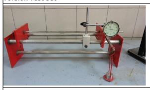
Finding properties such as shear modulus (G) and shear yield stress (tA) of materials by performing Torsion Test
